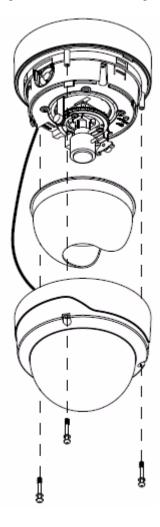
Figure 2-6 Attaching the Privacy Shield and Dome
